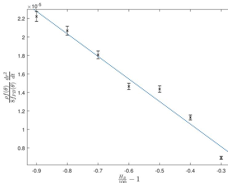
Figure 1: Evaporation rate as a function of humidity, the gradient of the line gives an approximation of the diffusion coefficient as  $2.44 \pm 0.48 \times 10^{-5} m^2 s^{-1}$
