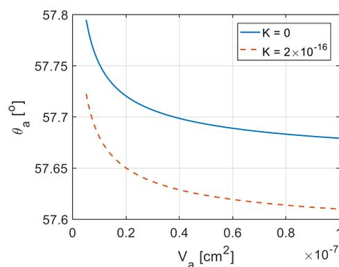
**Fig. 1. Static advancing of droplets on deformable substrates are lower to those on a non-deformable substrate**
